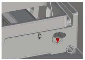
The main power switch is located on the left side the helmsman seat.
