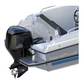
The engine should be in such a position so it wouldn't allow the screw to cavitate. Cavitation of screw reduces the engine efficiency and and in consequence the towing power. The excessive diving of engine introduces additional resistance of hull, which reduces the sailing speed.
