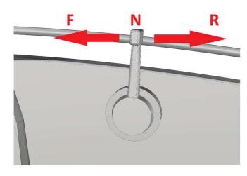
**N – neutral position** – safe position of throttle lever to start the engine.
