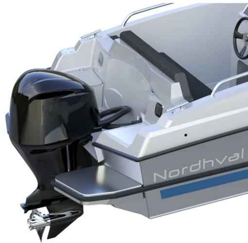
The engine should be in such a position so it wouldn't allow the screw to cavitate. Cavitation of screw reduces the engine efficiency and in consequence the towing power. The excessive diving of engine introduces additional resistance of hull, which reduces the sailing speed.
