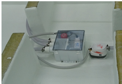
Automatic bilge pumps
