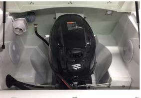
To drive the boat, you should apply the motor with the maximum power recommended by manufacturer of the boat – max. 44,7 kW. The engine might be with a long column.
