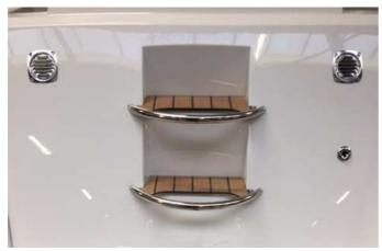
The end exhaust is mounted on the back wall of the stern.
