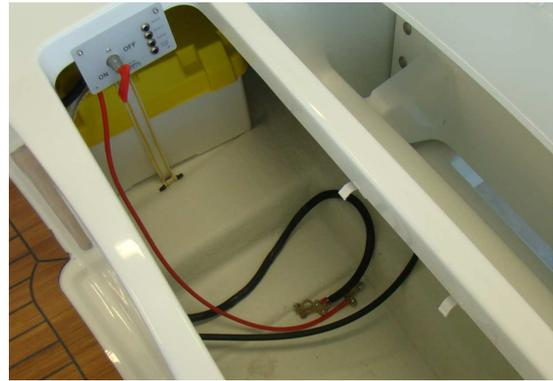
Photo shows the location for the battery including derived leads.
