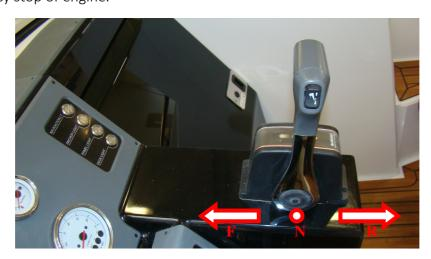
**N – neutral position** – the position of throttle lever to starting of engine.
