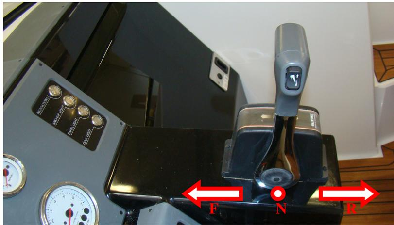
**N – neutral position** – the position of throttle lever to starting of engine.
