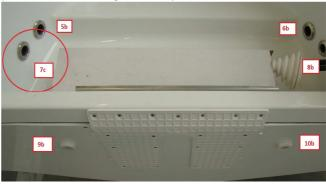
The outflow from the bilge with an automatic bilge pump to the engine compartment
