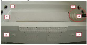
9 10 The outflow from the engine compartment on the outside of the transom
