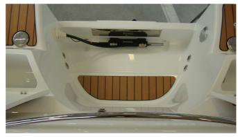
recommended by manufacturer of the boat – max. 128,7 kW. The engine might be with a long column.
