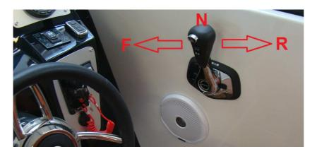
**N – neutral position** – the position of throttle lever to starting of engine.
