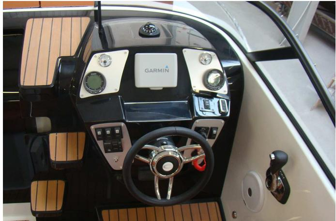
**The throttle changes the speed and the direction of driving screw.**
