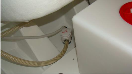
Hand bilge pump inside engine compartment
