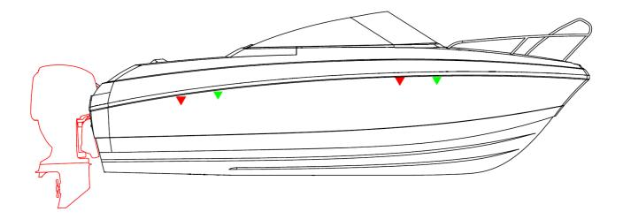
Red triangles marked places where you should put the lifting belts with engine.
