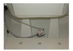
Hand bilge pump inside engine compartment
