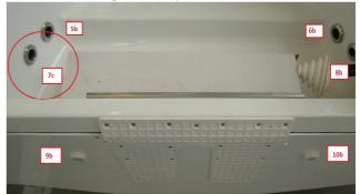
The outflow from the bilge with an automatic bilge pump to the engine compartment 8
