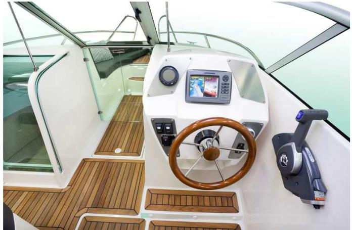
**The throttle changes the speed and the direction of driving screw.**
