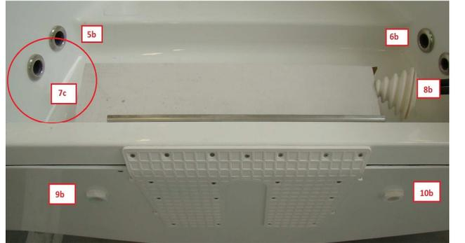
8 The outflow from the bilge with an automatic bilge pump to the engine compartment
