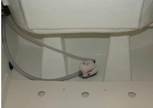
Hand bilge pump inside engine compartment
