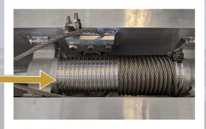
3.5 Inch Diameter Grooved Cable Winder vs 2.75 Inch
